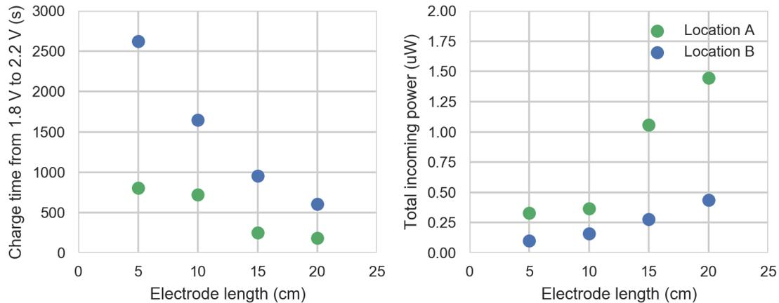
Fig. 6. Charge time and incoming power for different lengths of electrode.
