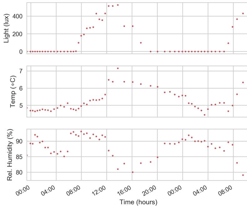
Fig. 13. Environmental parameters logged by our harvester and wirelessly streamed to a base station over a period of over 36 hours.
