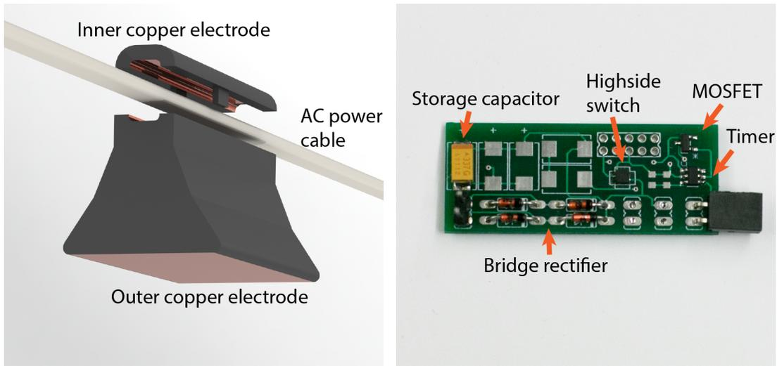
Fig. 2. (a) The CapHarvester (capacitive energy harvester) clamps on to a low-voltage power cable and harvests power without current flow. (b) Our power harvesting circuitry rectifies the capacitively coupled 60 Hz power line signal and stores energy in a capacitor with low leakage current. A high side switch, timer, and MOSFET added to the power management circuit control the attached peripherals.
