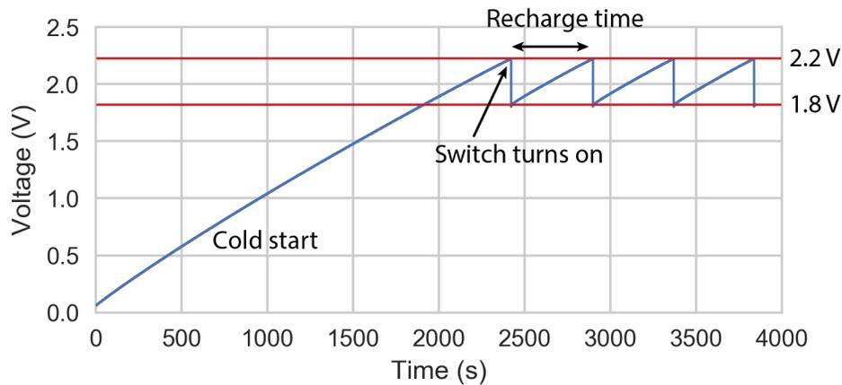
Fig. 5. When first installed, the harvester begins its cold start period. Once the storage capacitor reaches the trigger voltage of the high-side switch ( $2.21\text{ V}$  here), the switch activates and the device becomes active until the voltage drops to the lower cutoff voltage ( $1.8\text{ V}$  here). After that the recharge time of the device is significantly reduced.
