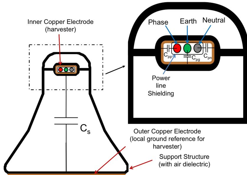
Fig. 3. Cross-sectional model of a power line having three conductors (phase, neutral, and earth). Each conductor has a primary capacitance ( $C_{pp}$ ,  $C_{pn}$  and  $C_{pg}$ ) with respect to the inner electrode and a secondary capacitance ( $C_s$ ) exists between the inner and outer electrodes of harvester.
