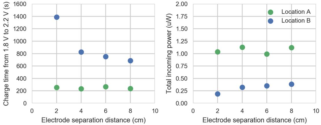
Fig. 7. Charge time and incoming power for different separation distances between the two electrode
