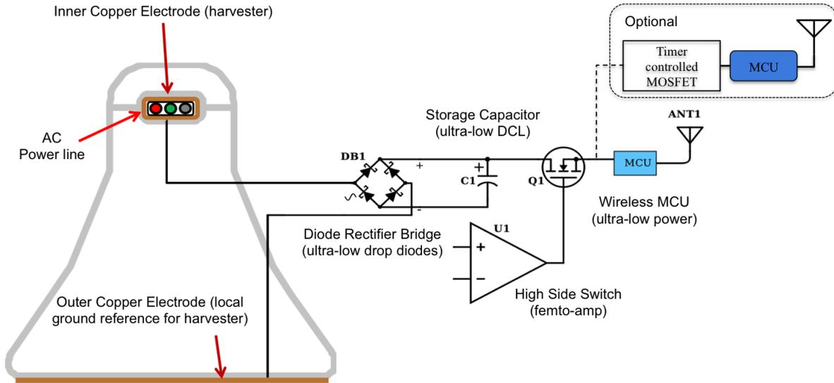
Fig. 4. The block diagram of our system, which consists of double-layer stacked capacitive electrodes, a diode rectifier bridge, a storage capacitor, a high side switch, and a wireless MCU for sensing applications. Optionally we also add a timer controlled MOSFET circuit to drive wireless MCU for continuous and event based sensing applications.
