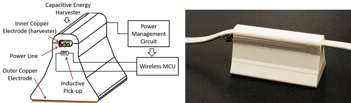
Fig. 9. (a) Block diagram of ApplianceTag showing inductive pick-up for sensing appliance state (on/off) and capacitive electrodes for energy harvesting (b) plot showing appliance state information (on/off) measured using ApplianceTag along with ground truth data from collected using current transformer
