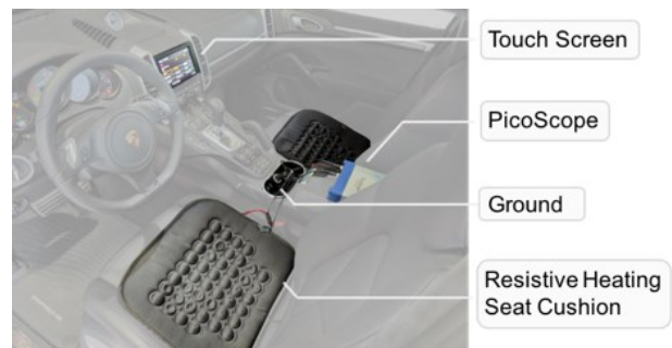
Figure 3: Carpacio data collection setup
