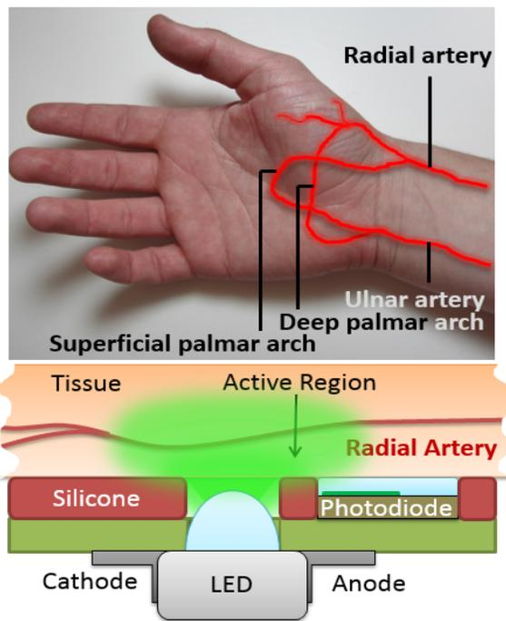
Figure 2. A low profile probe is obtained by use of reverse mount LED. Probe sits atop the radial artery just before the branches to the palmar arches.
